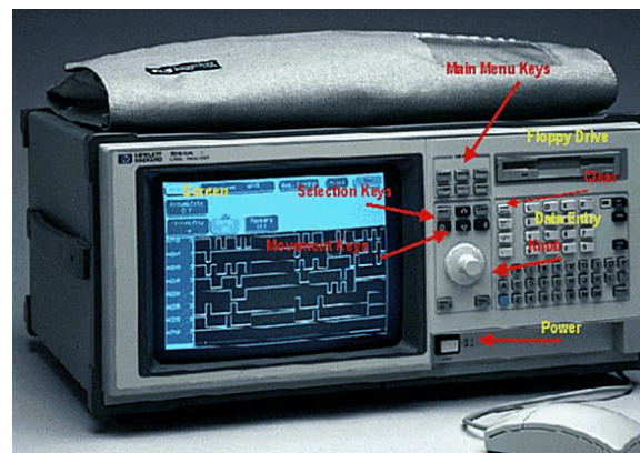
Figure 1.57 – The Logic Analyzer.
